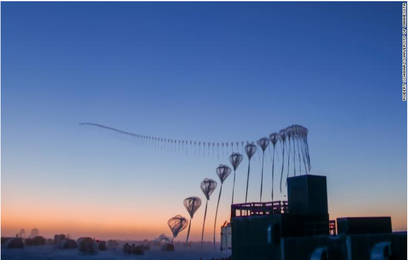
Picture Caption: A timelapse of weather balloons used to measure ozone.
